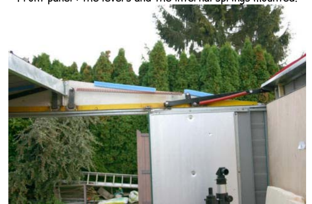
Then you can hang the external springs on both sides of panel.
